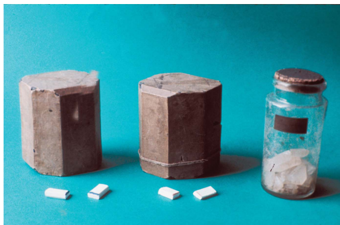
Figure 4 Pasteur's own cork models of a pair of crystals of sodium ammonium (2 R ,3 R )-tartrate and sodium ammonium (2 S ,3 S )-tartrate. In real crystals of these compounds, observation of the minor faces is more difficult than in the cork models. Courtesy of l'Institut Pasteur, Paris.
